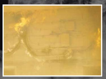
The plastic junction boxes melt within a few minutes. Shortly after, the cables burst with actual fire. The ceramic terminals ensure the continuous flow of current.
